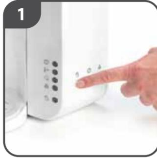
1 Press the cleaning mode button for 2 seconds to empty the tank (ensure a suitably sized receptacle is under the dispenser outlet to collect the water). Then press the filter volume reset button for 2 seconds to clear the memory.
