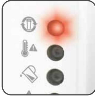
A red change filter warning light will illuminate when the filter needs replacing soon. If this light flashes, the filter must be changed immediately.
