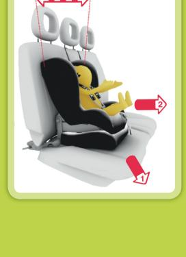
improve safety. In front and rear collisions our patented Pivot Link system stops your child being jolted so far forward – not only reducing the amount of force your child is subjected to, but reducing the odds of their head hitting the car interior.
