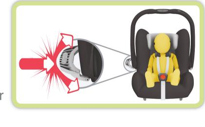
carriers. The D-SIP nearest the car door is then manually turned outwards and locked in place. Because this brings the point of impact closer, it reduces momentum first, and then disperses the energy through the entire carrier shell – away from your baby.
